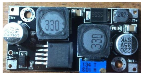
Figura 22: Conversor Buck-Boost DC-DC
