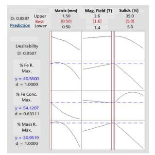
Figure 2 - Optimization graph for tests using WHIMS (Route 1).
