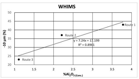
Figure 8 - Percentage of  $Al_2O_3$  in the fraction below 10  $\mu$ m of the concentration.
