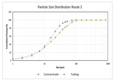
Figure 3 - Particle size distribution of the products obtained in the Route 2 tests.
