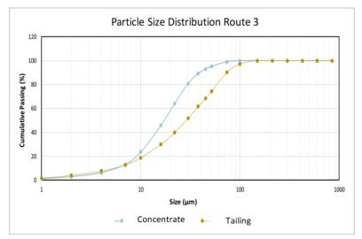
Figure 6 - Particle size distribution of the products obtained in the Route 3 tests.
