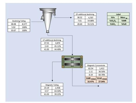
Figure 5 - Metallurgical balance Route 3.
