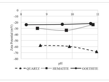
Figure 4 - Zeta potential of quartz, hematite and goethite, in the presence of sodium silicate, as a function of pH.
