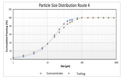
Figure 7 - Particle size distribution of the products obtained in the Route 4 tests.
