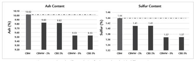
Figure 1 - Ash and sulfur analysis of coke produced with different mixtures.
