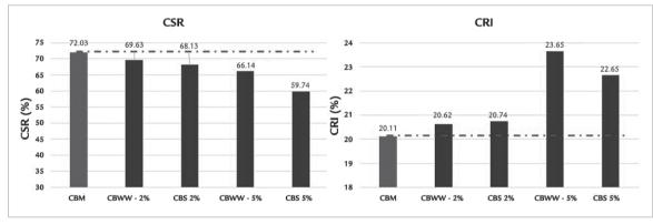
Figure 3 - CSR and CRI of coke produced with different mixtures.
