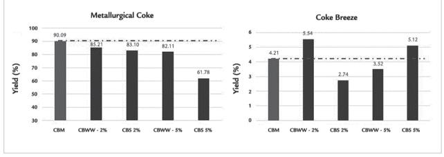
Figure 5 - Results of the fraction of metallurgical coke and breeze produced.
