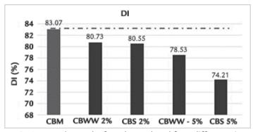
Figure 2 - Drum Index results for coke produced from different mixtures.
