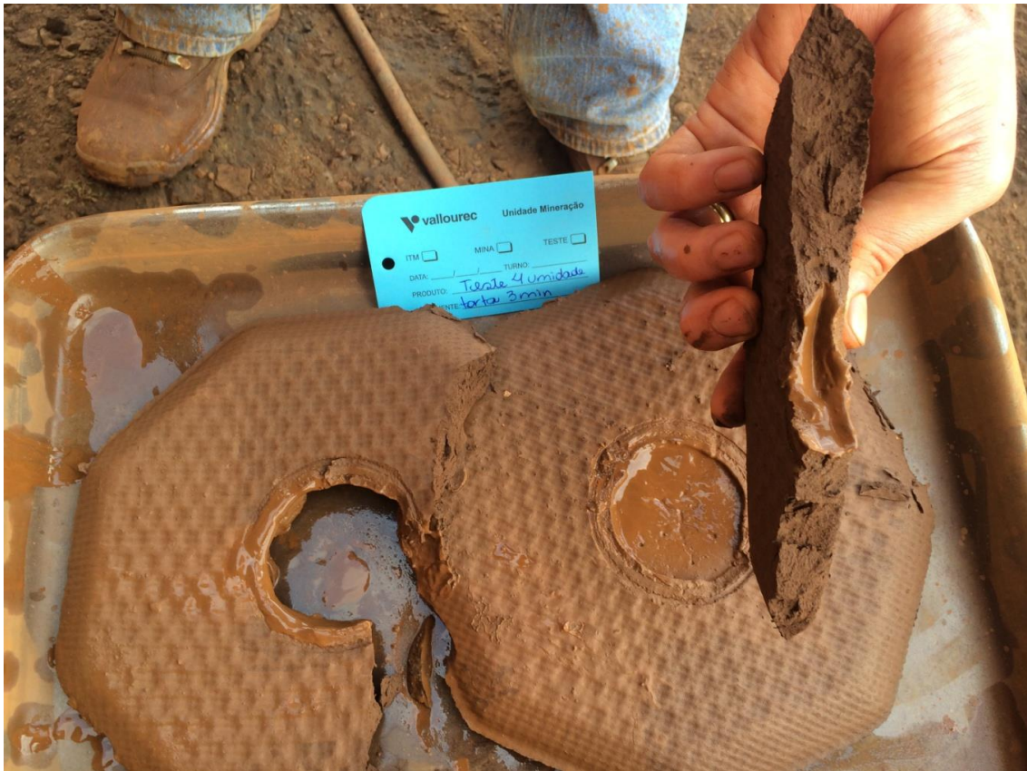
Fig. 7 Images of actual cake obtained from the laboratory filter. The best cake moisture was obtained for a cake thickness of 35 mm.
