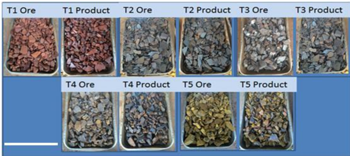
Figure 3 - Typologies before and after laboratory metallurgical tests. T1, T3 and T5 presented a significant increase in Fe content, due the elimination of LOI, SiO 2 , and Al 2 O 3 particles. Bar scale (300 mm)
