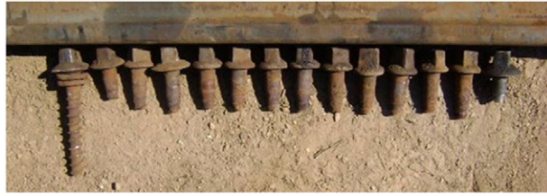
Fig. 1. In service failure of screw spikes.
