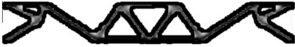
Fig. 16. Optimal setting by [6], nonlinear analysis of a slender plate attached at the vertices.
