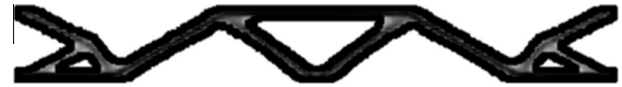
Fig. 15. Optimal setting by [6], linear analysis of a slender plate attached at the vertices.
