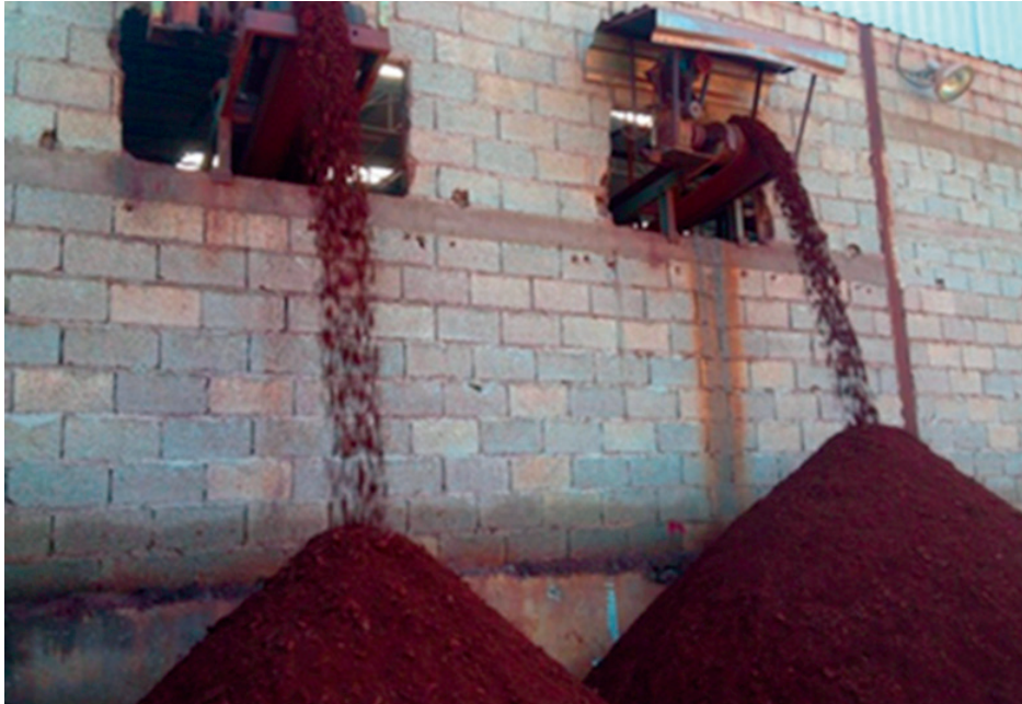
Figure 1 Waste dumps in construction by the conveyor belt method.
