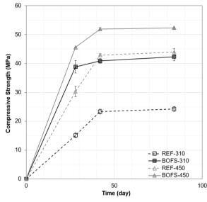
Figure 5. Compressive strength of the produced concretes
