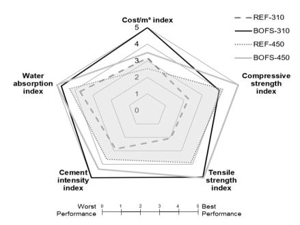
Figure 9. Radar chart of the technical, economic and environmental performance analysis of the concretes. Parameters are normalized, where 5 is the best performance and 0 the worst one.
