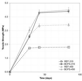
Figure 7. Tensile strength of the produced concretes
