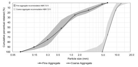
Figure 1. Particle size distribution for the coarse and fine aggregates
