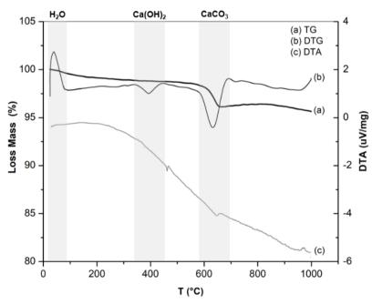
Figure 3. TG/DTA curves for the steel slag used
