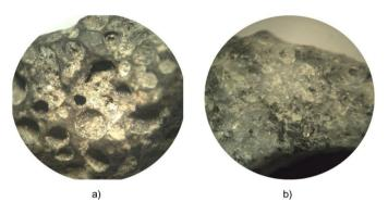
Figure 6. Microscopy images of aggregates, 15x magnification (a) steel slag (b) gneiss coarse aggregate
