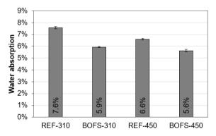
Figure 4. Water absorption of the concretes produced in the hardened state
