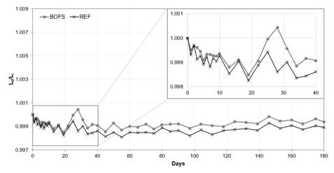
Figure 8. Expansibility of concrete specimens
