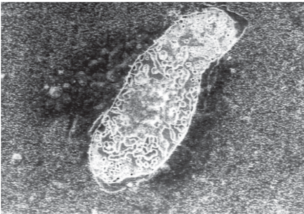
Figure 5. Observation of a spalled zone by SEM on the 439 steel oxidized at 950 °C in Ar-H 2 -H 2 O for 50 h (275×).
