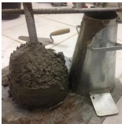
Figura 4.1 – Slump test.
