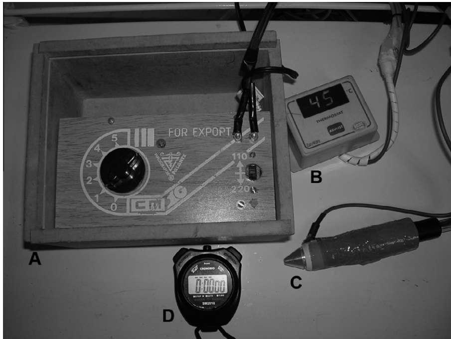
Fig. 1. The thermoalgesimeter built to assess heat-evoked nociceptive thresholds in mouse ears. A pyrography machine (A) was adapted with a thermostat (B) to control the heated metal extremity (C) at a maximum temperature of 45 °C. A chronometer (D) was utilised to record the time necessary for the withdrawal reaction.
