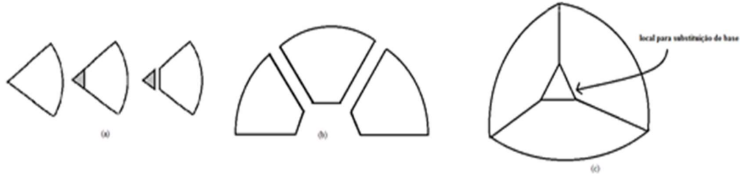
Figure 4: (a) mirror model in the form of circular sector and truncation of the circular sector; (b) planned kaleidoscope; (c) scheme of a generalized kaleidoscope and indication of the location for the placement of the base.
