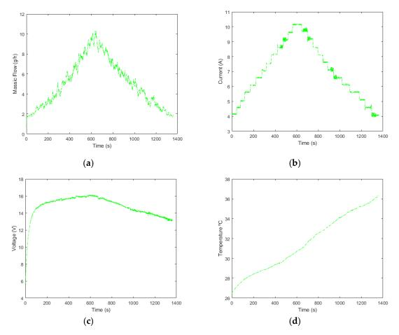
**Figure 4.** Results of (**a**) electrolysis gas mass flow (g/h) as function of time (s); (**b**)electric current (A) as function of time (s); (**c**) voltage (V) as function of time (s); (**d**) temperature ( $^{\circ}$ C) as function of time (s).
