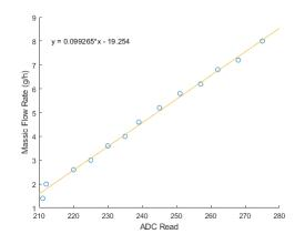
Figure 3. Winsen sensor calibration, F1012 model.
