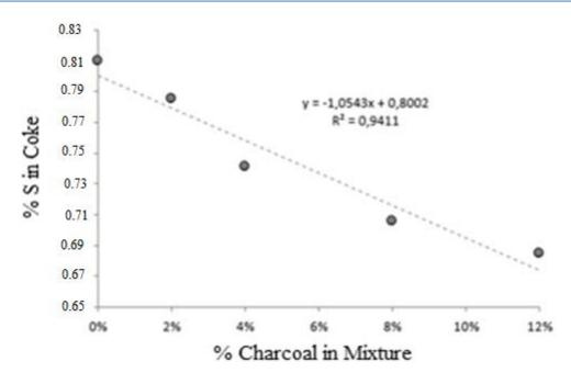
Figure 5: Effect of sulfur content in coke with biomass addition (Liziero, 2017)
