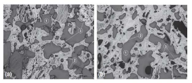
Figure 7: Biocogue optical micrographs: (a) coke with 10% charcoal; (b) coke with 10% charcoal and an additive. 1-Voids; 2-coke matrix; 3-particles of charcoal (Mathieson, 2015)
