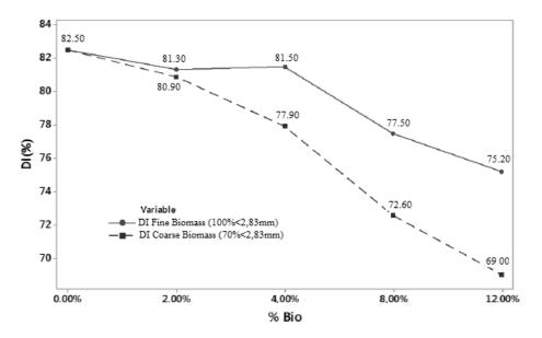
Figure 3: Evolution of DI with the addition of biomass (Silva, 2016a)
