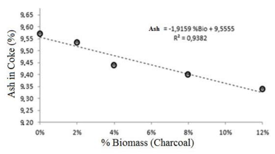
Figure 6: Ash behavior with biomass addition (Silva, 2016).
