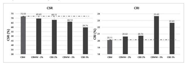
Figure 4: CSR e CRI of coke produced with wood and sawdust (Carvalho, 2021)
