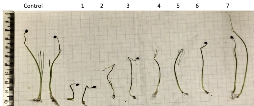
Figure 5. Allium cepa seedling development after watering non-contaminated soil with the soil-flushing eluted solutions. Numbers are indicative of the cycles carried out (bed volumes). Control set soaked with distilled water.
